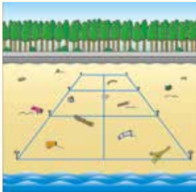
① Set up the survey blocks.
