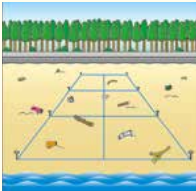
① Set up the survey blocks.
